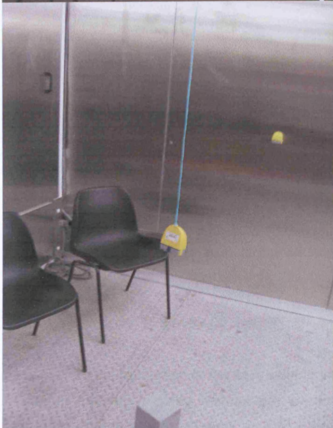
Figures 4-7: In these pictures, the dataloggers or Hobos can be seen, as well as their location inside the chamber. As it can be seen the hung Hobo is placed at the centre of the room. The picture at the top shows the arrangement of the chairs inside the room, at that point.
