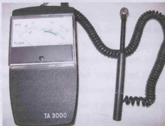
Figure 8: The anemometer used for the measurement of the air movement inside the chamber.
